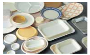
Board press mould products This system produces shallow, strong paper trays such as paper plates and food containers.
