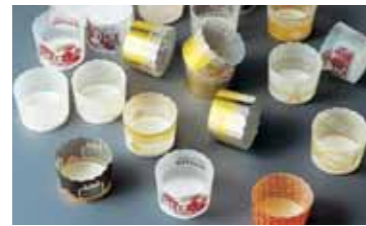
Tubular composite paper mould products This system produces jelly and mousse containers from composite paper. There are also many other possible applications.
